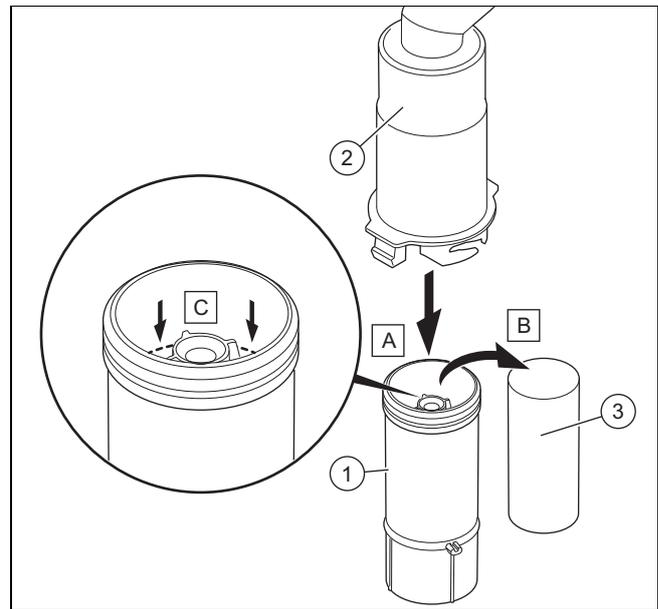
1. Unclip the lower section of the condensate trap (1) from the upper section of the condensate trap (2).
