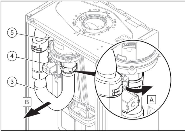
7. Remove the air intake pipe (3).
