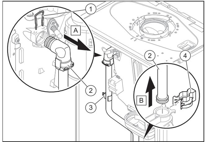
4. Remove the temperature sensor (3).
