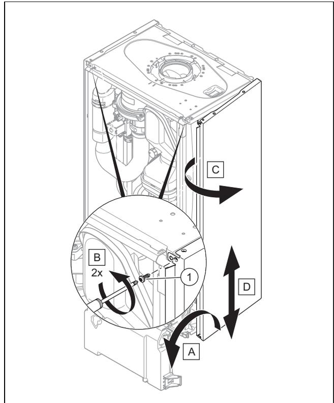
1. Hinge the electronics box forward.
