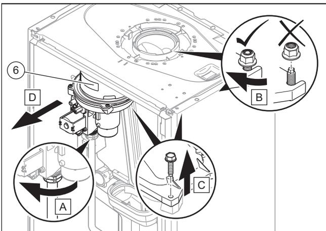
9. Remove the gas-air mixture unit (6).
